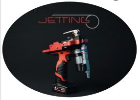
**TrigAir** — will blow 0.8 to 3mm cable into 3, 5, 7 and 8mm ducts for about 40-50m with no air and up to 500m with Air.
