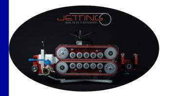
**V3** - will blow 4 to 40mm cable into 10 and 63mm ducts for about 40-50m with no air and 2500-3500m with Air.
