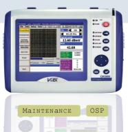
The CM3000 and CM3800 analyze Upstream and Downstream network performance for business and bundled services. Both instruments validate the effectiveness of DOCSIS 3.0 services, by testing up to eight downstream bonded channels and four upstream channels. The CM3000 is field upgradeable to a CM3800 via simple firmware upgrades.
