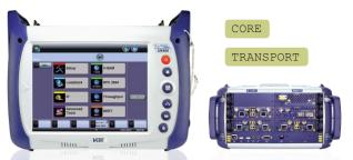
The robust UX400 Universal Expert is the most versatile portable multi-service transport test solution to offer test capabilities ranging from DS1/E1 all the way up to the latest 100GE network speeds, in a compact chassis with battery backup. Its modular architecture supports up to six independent test modules, in a multiuser environment.
